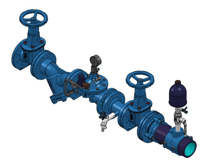
The HAWIDO must be installed horizontally with the valve cover upwards (other models available on request). We recommend that a gate valve and a dirt trap be fitted in front of the valve, as well as the mounting of a gate valve at the outlet.
